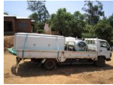
Left to right: Flat pack desludging kit, Membrane pump, Kit mounted on truck
